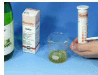
Dip sulphite test strip into sample for 1 second and compare it with colour scale
