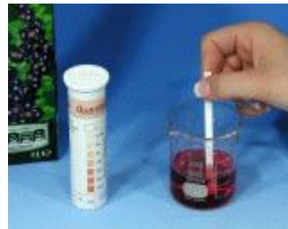
Dip the test strip 1 second into the juice
