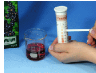
Compare the test field with the colour scale on the tube
