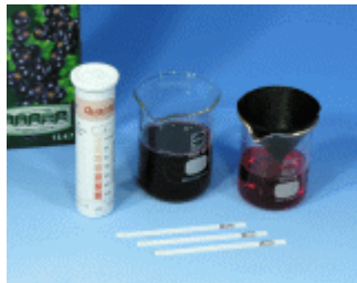
To test currant juice filter with activated charcoal paper
